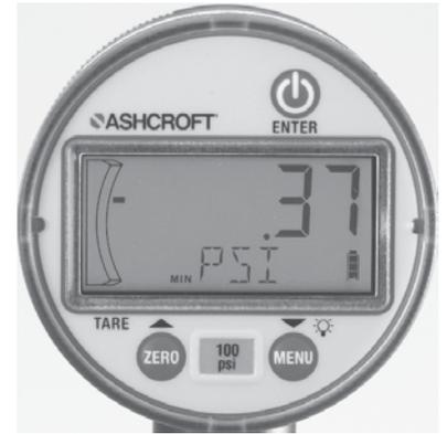
**Note:** Clearing Minimum / Maximum values will reflect a blank display except for the associated Min. / Max. icon and battery indicator.
