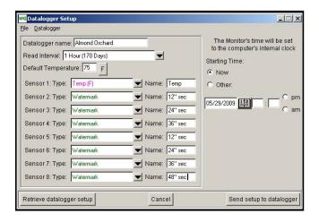
The WATERMARK Monitor is user-programmed for the individual characteristics of the site being monitored using WaterGraph Software WG3 for 900 Series Monitors.
