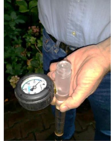
Step 4: screw cap firmly on the shaft
