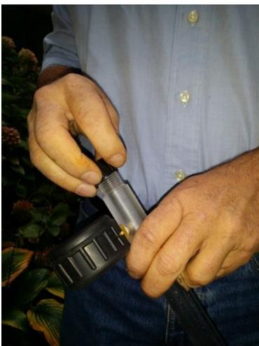
Step 2: fill Tensiometer completely with water
