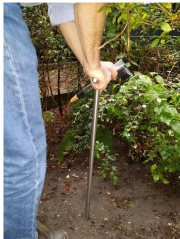
Step 6: Push Tensiometer firmly but with caution to the bottom of the hole. The needle of the
