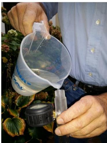
Step 3: Remove trapped air from Tensiometer with the service pump (included). This process must be repeated several times until no more air bubbles come from the inside of the Tensiometer and the Manometer. After this fill the Tensiometer again with water to the brim.
