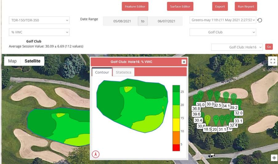
Fig. 3. 2-D Mapped Readings and Contour Plot in SpecConnect
