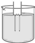
1. A clean glass or plastic container. The container must be at least 10cm (4”) wide and 5.08cm (2”) longer than the length of the TDR rods.
