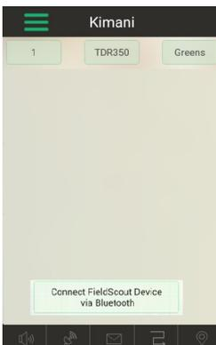
Figure 1a. Bluetooth Connect button (grid)
