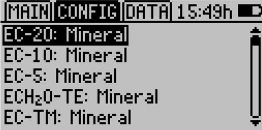
To modify a sensor's calibration type, press **ENTER**. You can choose a preset soil calibration type or create your own (See creating a Custom Calibration). To change the soil calibration type, press **ENTER** when the medium option is selected. You can view the calibration coefficients by pressing **ENTER** when the coefficients option is highlighted. Press **SAVE** to save your calibration preference or press **ESC** to exit without saving changes.
