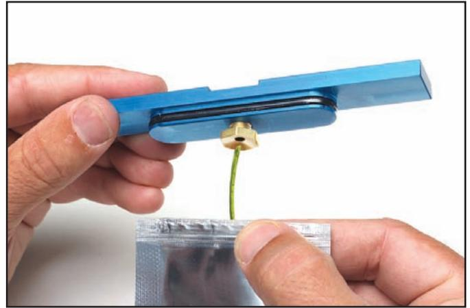
4. Turn Compression Gland Screw clockwise to tighten the gasket around the sample. This depends upon which lid is being used. With the Small Lid, the Compression Gland Screw is made of brass and is on the inside edge of the lid. The Large and Grass lid have an anodized blue Compression Gland Screw that is external.
