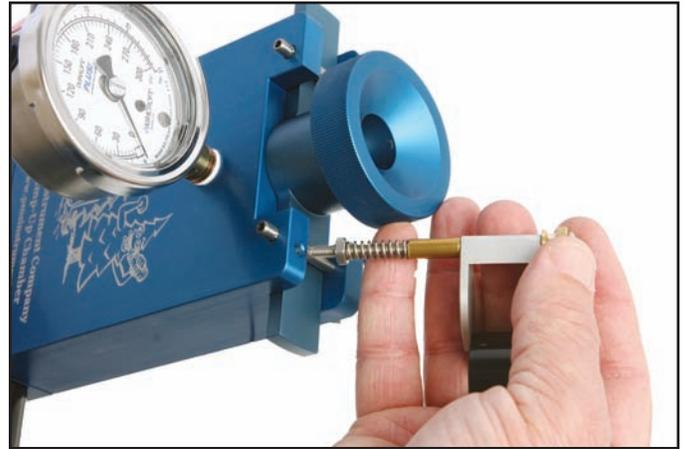
2. Screw into the mounting hole until the nut touches the chamber.
