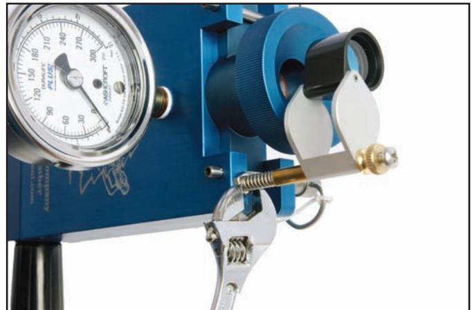
4. Use the knurled brass nut to adjust the focal point of the lens appropriate for your vision.
