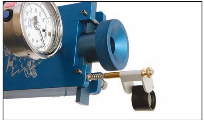
3. Use a wrench to tighten the nut into place so the Eye Lens is secure.
