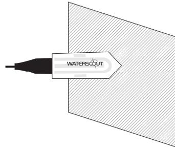
during installation. To limit the effect of water moving vertically through the soil profile, the sensors should be installed so the flat face is perpendicular to the soil surface. For the same reason, if sensors are installed at multiple depths, they should be offset from one another.
