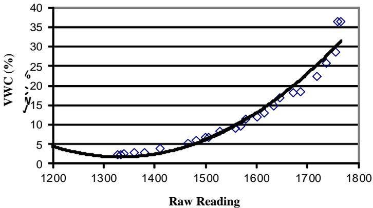
A calibration curve can also be obtained by gradually wetting a pre-measured amount of soil with known increments of water. Care must be taken to return the soil to its original bulk density before a sensor reading is made.
