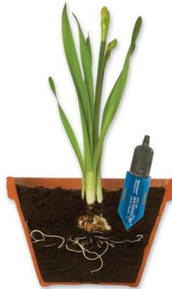
The SMEC 300 is most sensitive to the soil adjacent to the sensor. Therefore, good contact between the soil and sensor is important. Stones and air pockets next to the sensor will affect the accuracy of the readings. Because it is sensitive to differences in dielectric permittivity, care should be taken not to install the sensor in or near metal.
