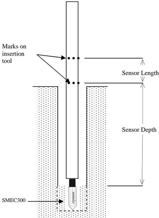
and that the sensor is being installed to the desired depth. The access hole should then be carefully backfilled with native soil and tamped down to eliminate air pockets.
