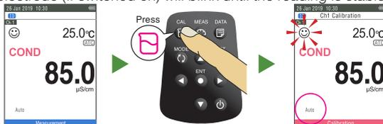
4. Press ENT button to confirm the conductivity reading. To abort calibration, press MEAS button.
