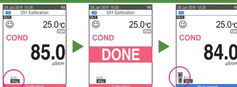
5. Repeat step nos. 1 to 4 to perform calibration with the next standard solution(s).
