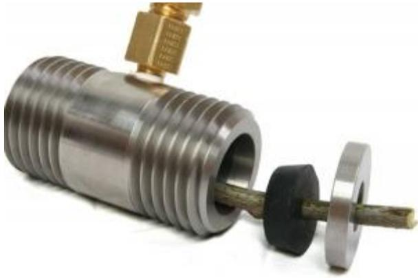
The rubber gaskets slide down the sample and seat inside the chamber.
