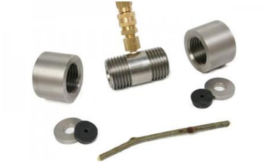
The cavitation chamber feature of this instrument is used to simulate cavitation of xylem vessels in plants under stress. A plant stem, limb or root is introduced into the Cavitation Chamber and a head of water is connected to the sample to measure water conductivity. The chamber is then pressurized to “seed” air into the xylem. It can be used to establish vulnerability curves in plants or to continue [research](#) in the area of xylem cavitation.
