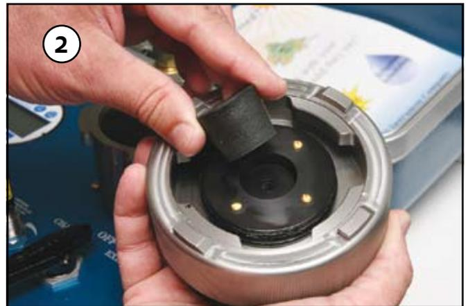
*Insert a solid rubber gasket into the lid*
