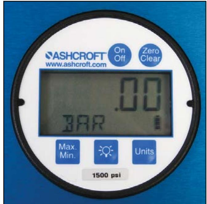
If the ON/OFF button is pressed and held for three seconds, a menu will appear, which can be scrolled through by pressing the ON/OFF button. The menu will offer the following selections, which will be blinking to indicate a selectable option:
