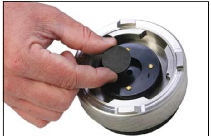
Turn control valve to **CHAMBER** position and pressurize the chamber. Adjust **Rate Valve** until pressure in the chamber increases at the desired rate. ½ Bar per second is a recommended rate of increase. Rate may be changed at any time, even while pressurizing a sample.
